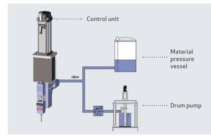
The vectodis metering system is suitable for processing single-component media. The material is discharged in shot or bead form. The material is taken from the original container via a feed pump and fed to a piston metering unit with a servo motor. A material pressure regulator keeps the input pressure at the piston metering unit constant.
